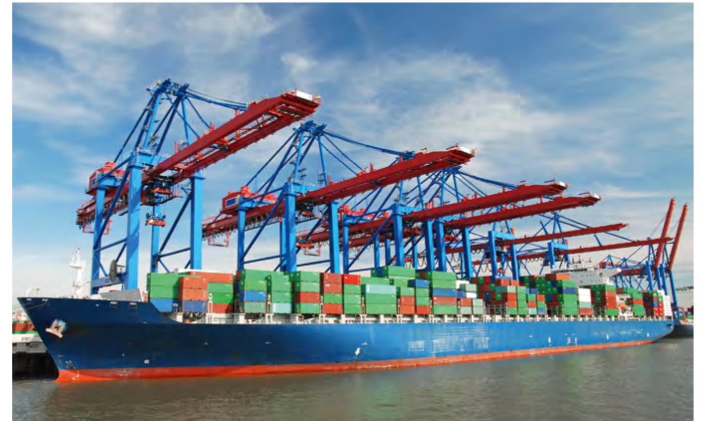
Gantry crane for loading containers at ports
