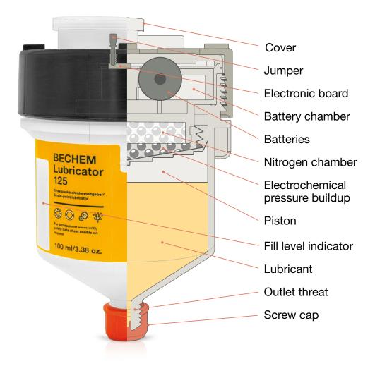
The BECHEM lubricator can be used independent of the position. After expiration of the operating time the lubricator will be replaced by a new unit.
