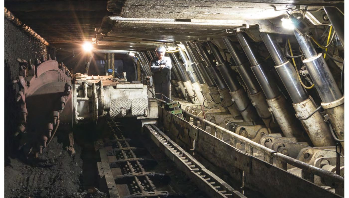
Hydraulic shield support with integrated chain conveyor and shearer
