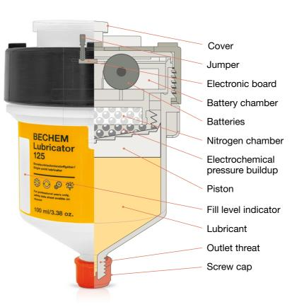
The BECHEM lubricator can be used independent of the The housing is weatherproof, corrosion resistant and offers position. After expiration of the operating time the lubricator will be replaced by a new unit.
