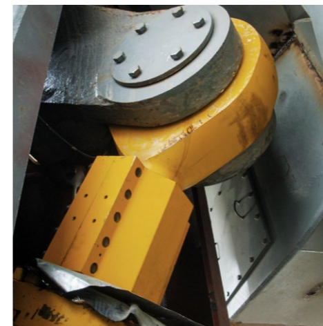
Tension rod bearing of a vertical roller mill
