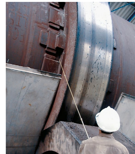
Application of Berulub VPN 13 Ringlub with the BECHEM Compression sprayer
