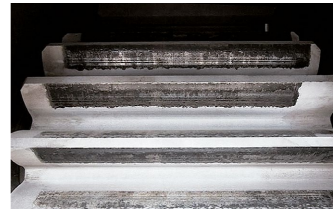
Flanks of a kiln gear drive before the running-in
