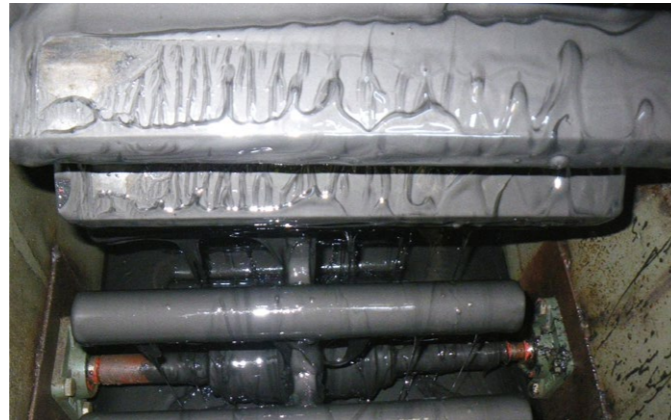
Open gear drive with paddle wheel lubricated by Berulit GA 2500 Fluid
